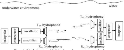
Figure1: Block diagram of full duplex active sonar communication
