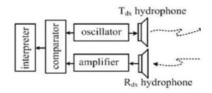
Fig2: Block diagram of half duplex active sonar communication
