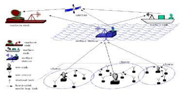
Fig4. Architecture of acoustic underwater communication
